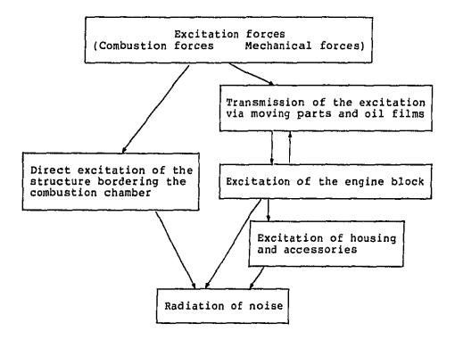
Thus the reduction of noise as a result of taking action on the engine itself can be concerned with the exciting force (explosion or combustion and the associated mechanical forces such as those due to side slap of the piston), with the transmission of that force via the moving parts and oil films or with the mechanical and acoustical response of the radiating structures involved (engine block, housing and accessories). II3.1. ACTION CONCERNING THE EXCITING FORCE
